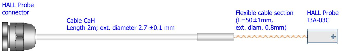
Figure 3. Dimensions of the I3C-03C Hall Probe and Cable (Module H).
