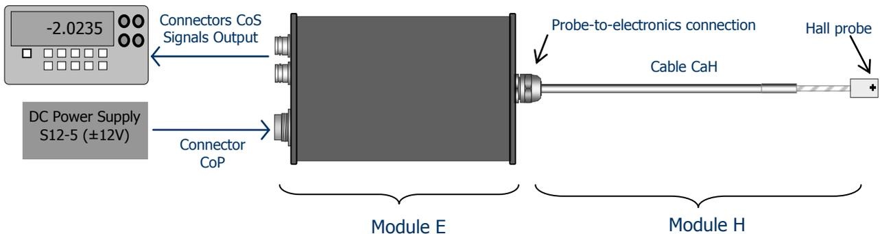
Figure 1. Typical measurement setup with a SENIS magnetic-field-to-voltage transducer with integrated 3-axis Hall probe (module H) and electronics (module E, encapsulated in the box type B)
