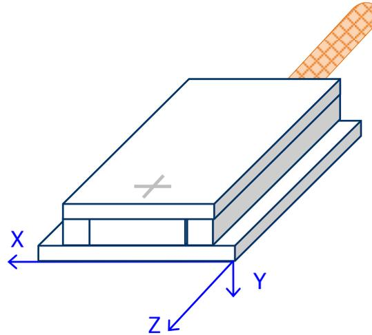
Figure 4. Reference Cartesian coordinate system of the SENIS I3A-03C Hall probe.
