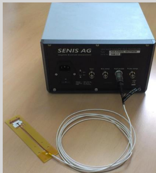
The SENIS Hall probe transducer used at MAX IV Laboratory
