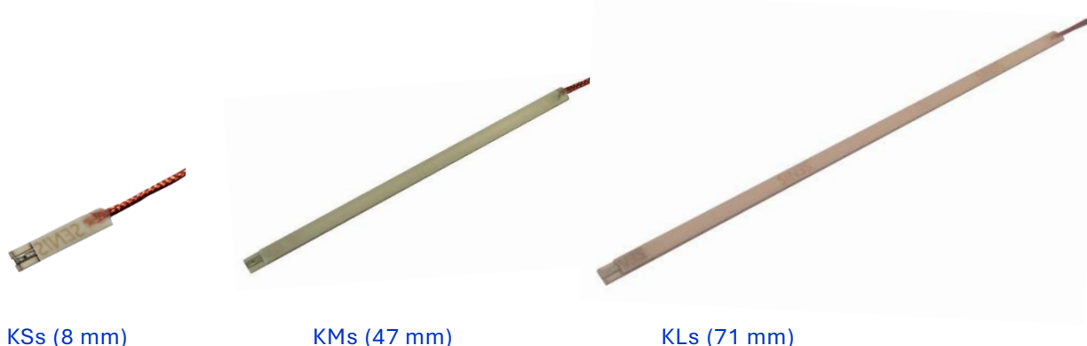
Figure 1: Photos of the 3-axis Hall probes type KSs, KMs and KLs
