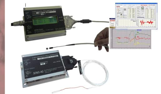
Arnold Magnetic Technologies AG (<u>www.arnoldmagnetics.com</u>) integrated at their facility in Switzerland SENIS 3MH3 digital Teslameter in their self-made magnetic scanner for accurate 3-axis magnetic field mapping of permanent magnets
