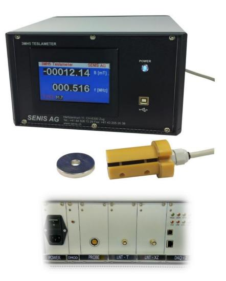
**Bruker BioSpin AG**, Switzerland (<u>www.bruker.com</u>) uses the Low Noise & High Resolution Teslameter / Gaussmeter for high accuracy measurements of high magnetic fields up to 20T. The magnetic resolution of **SENIS 3MH5** is less than 2ppm and accuracy better than 100ppm.
