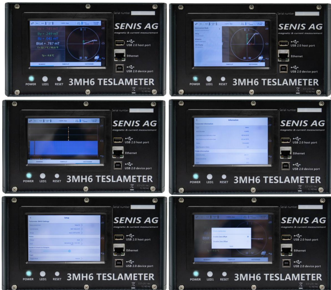
Figure 4: Visualization Modes (Numeric, Plot, Histogram) and Setting possibilities; External/Internal Triggers; Data Recording; Auto range; Zeroing; Min/Max; Hold reading;
