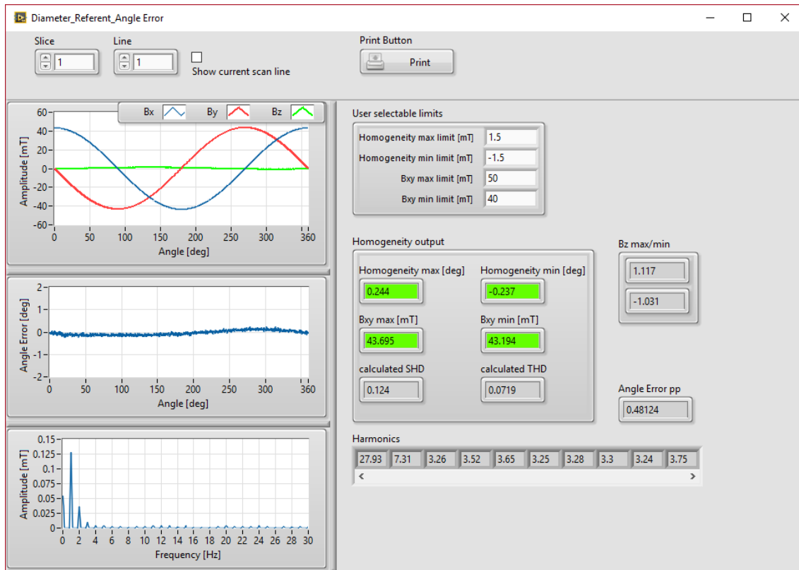
Figure 13: Dipole Magnet Analysis - App: GOOD/BAD Analysis based on the thresholds of Angle Error (Homogeneity), Min/Max values of the magnetic field components and Fourier Analysis
