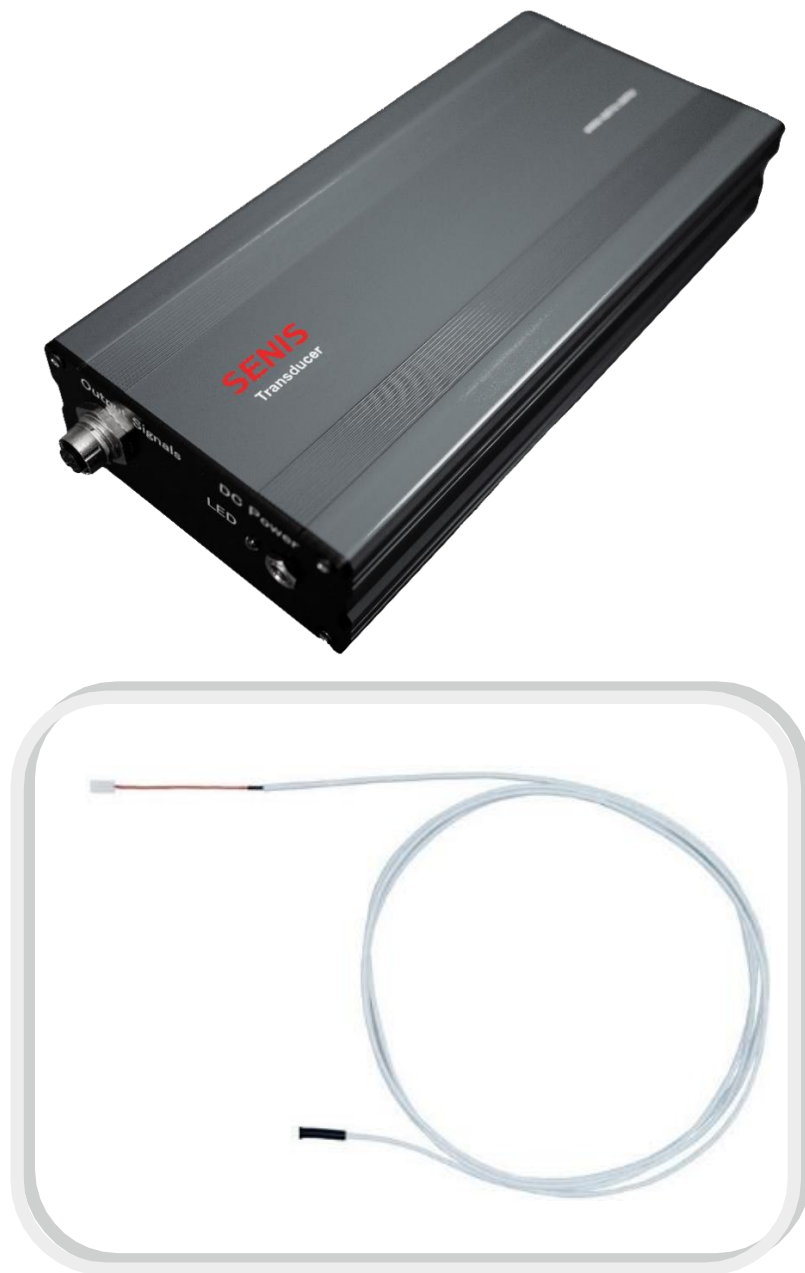
Figure 2: Photo of 3-axis magnetic field transducers H3B with hybrid 3-axis Hall Probe. Only one probe cable variant is available - flexible shielded white cable, OD 2.7 mm.
