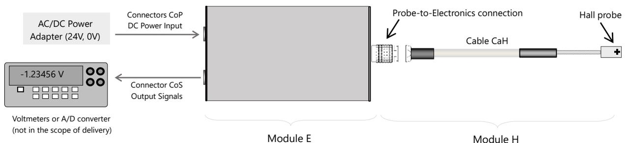
**Figure 1:** Typical measurement setup with a SENIS magnetic-field-to-voltage transducer with integrated 3-axis Hall Probe (Module H) and Electronic (Module E)
