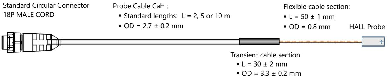
**Figure 3:** Dimensions of the Hall probe-to-transducer Cable CaH
