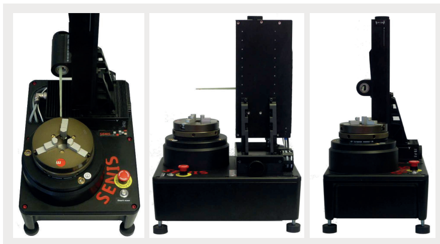
Figure 1: True 3-axis MMS-2A-ROT Magnetic Field Mapper for Rotational Scanning
