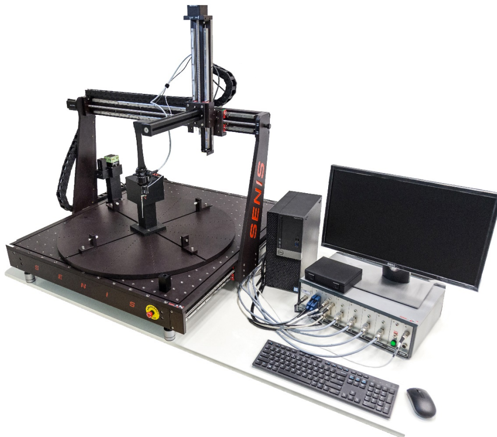
Figure 3: Full system with mapper, electronics and personal computer
