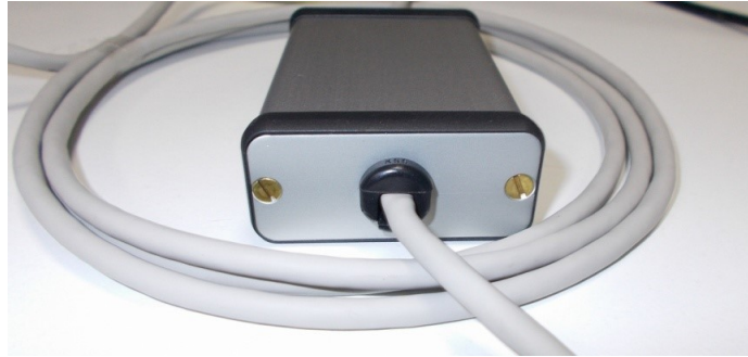
Figure 6: Cable extension electronic interface: the cable length from 2m to 40m and more
