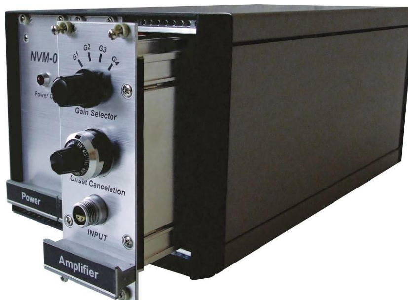
Figure B: Removing "Amplifier" module from electronic box
