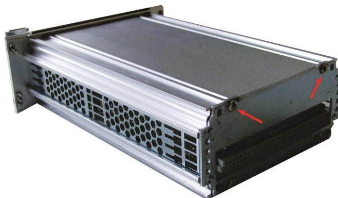
Figure D: Removing top cover from "Amplifier" module.
