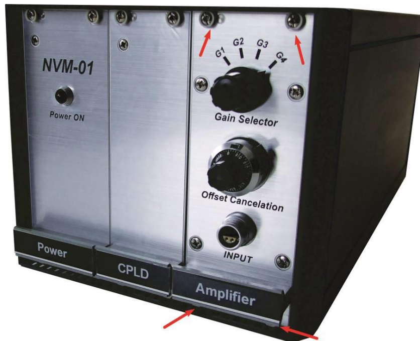
Figure A: Removing "Amplifier" module from electronic box
