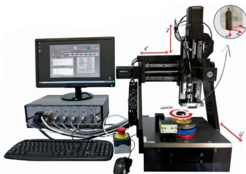
Fig. 11: The new Magnetic Field Mapper consists of four main parts: (a) the mechanical part, (b) the Hall Probe (or any other probe – as shown in Fig. 12), (c) an electronic box with digital signal processing, motor drives, encoder control, and power supply; (d) and a PC and Software for measured data acquisition, visualization, and analysis.
