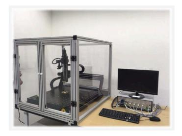
"Customers like our product for two reasons; the first one is that SENIS Mappers can measure all three components of magnetic field with unprecedented accuracy and repeatability very close to the magnet surface and in small gaps. The second reason is that our mapper software is very user-friendly and offers different types of data visualisation."
