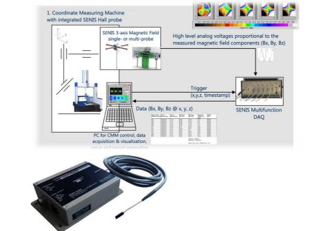
**Technetics Group** (<u>www.technetics.com</u>) utilizes **SENIS Magnetic Field Scanning System** for QA. SENIS and Technetics successfully integrated the SENIS magnetic field mapping system into a Zeiss CMM (Coordinate Measuring Machine).
