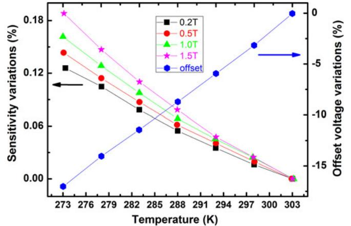
Fig. 7. Temperature dependence of the sensitivity and offset voltage.
