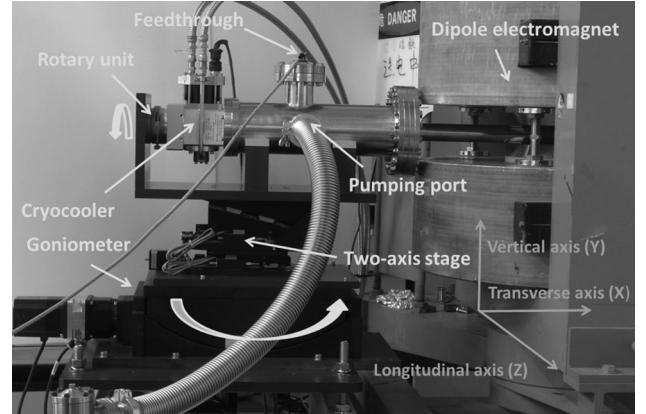
Fig. 1. Setup of the low temperature Hall probe calibration system.
