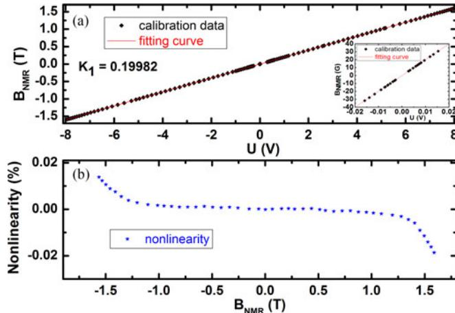
Fig. 8. (a) Field calibration data and (b) nonlinearity of the SENIS probe.
