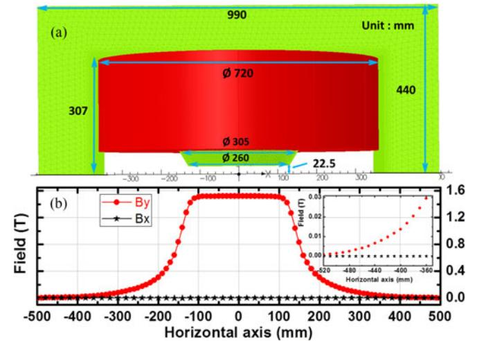
Fig. 3. (a) The upper part of the dipole electromagnet simulation model and (b) the field distribution along the horizontal axis.
