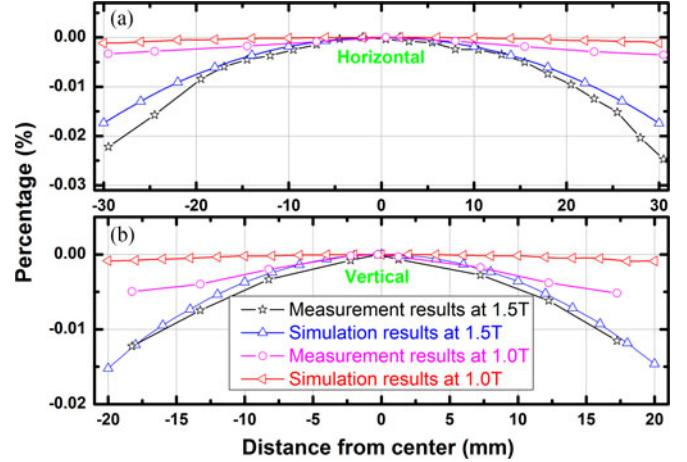
Fig. 5. Dipole magnet good field region as determined by measurements and simulation in (a) the horizontal and (b) vertical directions.
