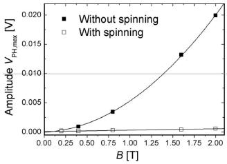
Fig. 9. Measured planar Hall voltage of the horizontal Hall plate without and with the application of the spinning-current method. A similar result is also obtained for the vertical Hall devices.
