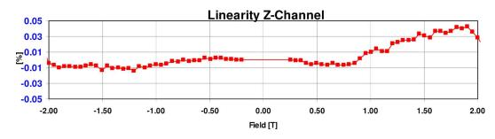
Fig. 12. Transducer nonlinearity error as a function of the measured magnetic flux density in the range  $\pm 2T$ .
