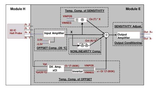
Fig. 10. Functional block diagram of the analog electronic module E. Only the signal path for channel X is shown. The same also exists for Y and Z.
