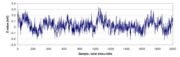
Fig. 13. Time dependence of the offset voltage of channel X. Abscissa: the order number of the samples. Ordinate: the offset voltage in millivolts.
