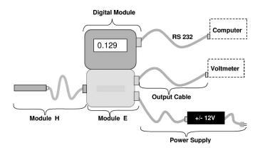
Fig. 1. Structure of the teslameter. An analog teslameter (transducer) consists of the modules H (Hall) and E (electronics), which are connected to an external power supply and voltmeter. The digital version includes an RS232 interface.
