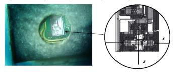
Fig. 5. Photo of the window of the probe that was shown in Fig. 3. The inset shows the magnetic-sensitive part of the integrated Hall probe. The field-sensitive point is located at the crossing point of the axes x and z.
