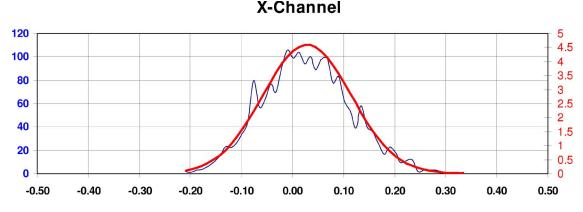
Fig. 14. Histogram of the values from Fig. 12 and the corresponding approximation by a Gaussian distribution. The standard deviation is about 83  $\mu$ V, which corresponds to 17  $\mu$ T.
