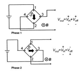
Fig. 11. Spinning-current method for the cancellation of the offset voltage of a Hall device. A Hall device is alternatively biased in two orthogonal directions. Then, the offset voltage due to the resistance asymmetry  $\Delta R$  changes its sign, whereas the Hall voltage does not change. By averaging the output voltages of the two phases, one can cancel out the offset voltage.
