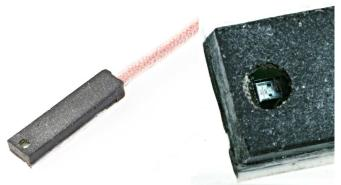
Fig. 3. Thee-axis Hall probe with a window. The magnetic-sensitive region of the integrated Hall sensor is visible through the window, which allows for precise positioning of the probe. The dimensions of the probe are 4 mm  $\times$  2 mm  $\times$  16 mm.
