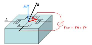
Fig. 7. Planar Hall effect. A magnetic flux density vector  $\boldsymbol{B}$  acting on a Hall device can be decomposed into a normal component  $\boldsymbol{B}_n$  and a planar component  $\boldsymbol{B}_p$ . The normal component  $\boldsymbol{B}_n$  produces a "normal" Hall voltage  $V_H$ . The planar component  $\boldsymbol{B}_p$  produces the planar Hall voltage  $V_P$ . The total output voltage is the sum of the normal and the planar Hall voltages.
