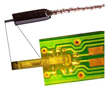
Fig. 4. World's smallest three-axis Hall probe. The thin tip of the probe is a part of the silicon integrated Hall sensor chip, which is not encapsulated. The dimensions of the naked silicon tip are 0.5 mm  $\times$  0.55 mm  $\times$  3 mm. The magnetic-sensitive point is only 0.15 mm away from the tip end.
