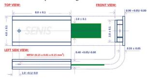
Fig. 4b. The dimensions of standard ceramic package of SENIS three-axis Hall probes (length x width x thickness): 8.0mm x 4mm x 0.9mm.
