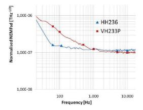
Fig. 3. Measured noise-equivalent magnetic field spectral density of the SENIS' Hall devices [4] implemented in 0.35μm CMOS technology, normalized to biasing power of 1mW. HH236: horizontal Hall device
