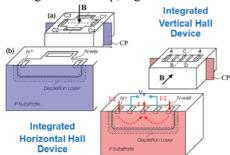
*Fig. 1. Integrated horizontal (left) and vertical (right) Hall devices in a single silicon chip.*
