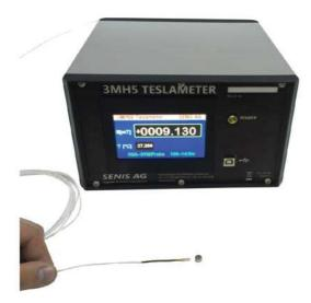
Fig. 8. SENIS High-Accuracy Teslameter with a very thin three-axis Hall Probe encapsulated in ceramic package
