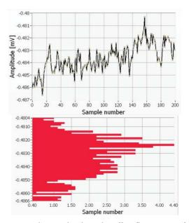
Fig. 7. The graphs show the offset fluctuation of the SENIS Low Noise Transducer, with the Hall probe placed in a Zero Gauss Chamber, over a time period of 10 seconds. The upper graph shows the offset in the time domain and the lower graph shows the related histogram. The sensitivity of the transducer is 1.25V/T and full scale 2T (FS). The measured fluctuation is  $5\mu Vp$ -p. This corresponds to the magnetic resolution ( $5\mu Vp$ p/1.25V/T)/2T = 2ppm(p-p)(FS).
