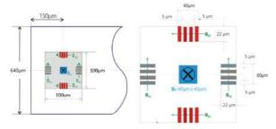
Fig. 2. The spatial distribution of the Hall devices of Fig. 1 on the Hall probe chip. The novel SENIS integrated Hall probes have the magnetic field sensitive volume) of 100μm x 10μm x 100μm (By: 45μm x 5μm x 45μm; Bx and Bz: 100μm x 10μm x 100μm).
