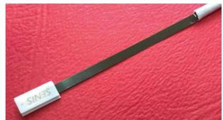
*Fig. 4a. Photograph of the standard ceramic package of SENIS three-axis Hall probes.* This package is suitable for the temperature range -55°C to +155°C.
