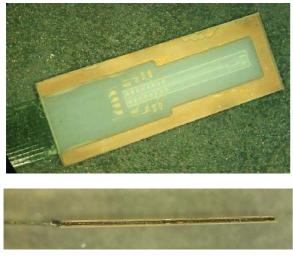
Fig. 5a. Photograph of the ultra-thin ceramic package of SENIS three-axis Hall probes. The dimensions (length x width x thickness): 8.0mm x 3mm x 0.25mm. This Hall probe is suitable for the industrial temperature range from -20°C to +85°C.
