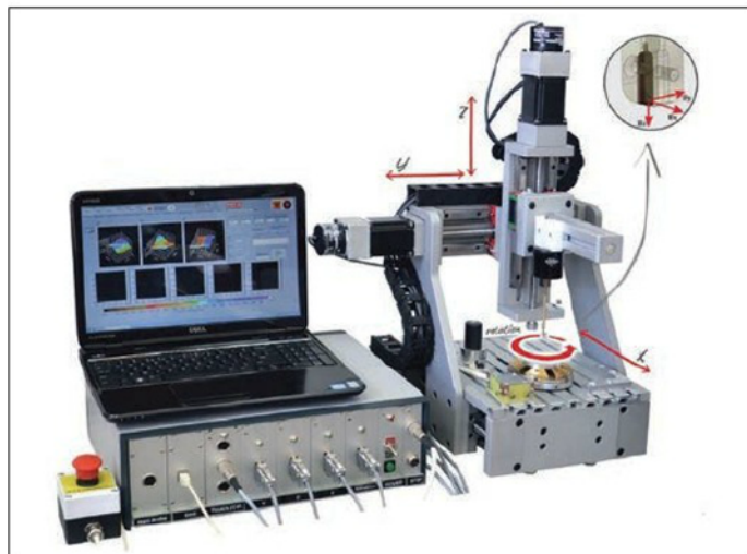
Figure 1. SENIS Magnetic Field Mapper consists of four main parts: (a) the mechanical part (the moving platform with three linear modules and the rotary stage); (b) the Hall Probe mounted on the Touch sensor; (c) the electronic box with digital signal processing, motor drives, encoder control, and power supply; (d) and a PC and Software for measured data acquisition, visualization, and analysis.
