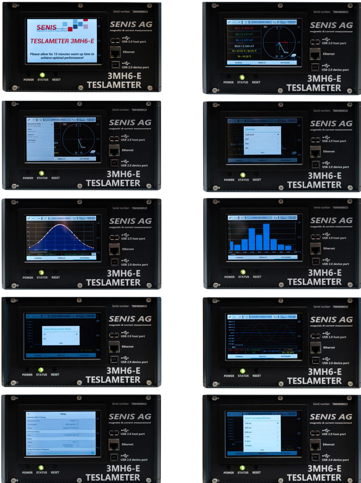
Figure 6: Visualization Modes (Numeric, Time-plot, Histogram) and Setting possibilities: External/Internal Triggers; Data Recording; Auto range; Zeroing; Min/Max; Hold reading; Sampling Rate; Averaging Rate; Storage interval.
