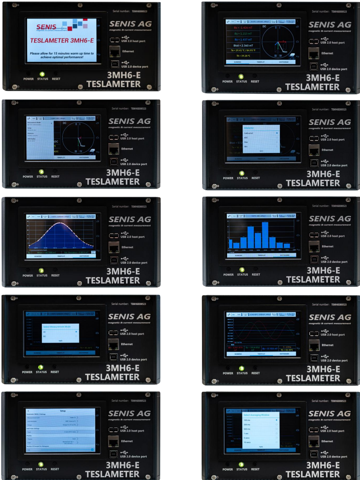
Figure 5: Visualization Modes (Numeric, Time-plot, Histogram) and Setting possibilities: External/Internal Triggers; Data Recording; Auto range; Zeroing; Min/Max; Hold reading; Sampling Rate; Averaging Rate; Storage interval.
