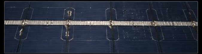
GOOD SOLDER CONNECTION
