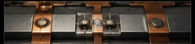
GOOD WELD CONNECTION
