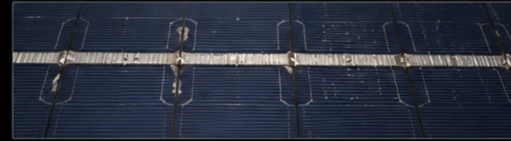
GOOD SOLDER CONNECTION
